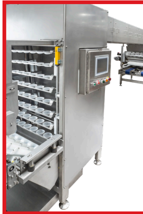
3. TOWER & PROOFER Tower with control panel and proofer
